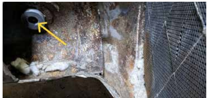
Rear pressure pickup of DPF
