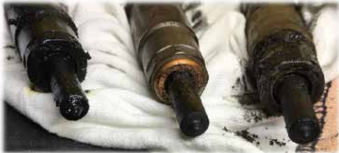
Failed injector washers
