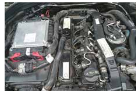
Pic 6 Mercedes converted Delphi piezo to electromagnetic
